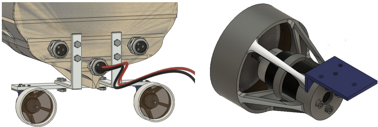
Figure 7: CAD of Full Motor Assembly Mounted on Hull (Left), Motor Assembly (Right)
