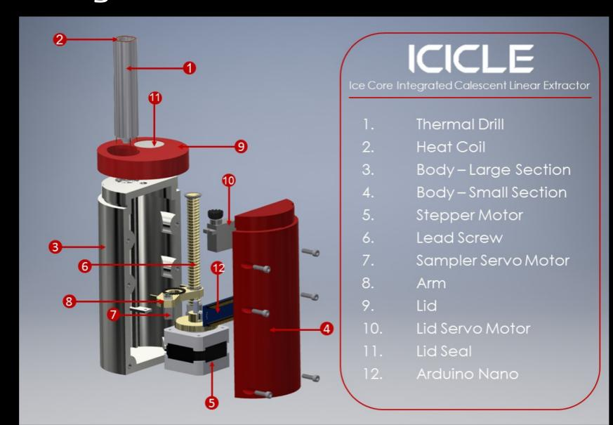
The team sought to find a design that met the volumetric requirement for sample retrieval, while ensuring the ICICLE would interface seamlessly with the JPL Buoyant Rover. ICICLE takes an input of 12V to actuate and heat a thermal drill which retrieves cylindrical ice samples of NASA's specified dimensions. The thermal drill allows for optimal under ice sample retrieval with a minimal administered buoyant force due to the efficiency of the thermal collection method.
